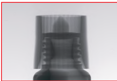
Sample is too far away from the X-ray source, low magnification
