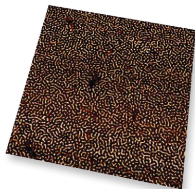
Closed-loop phase image revealing the micro-phase separation in a poly(styrene-b-butadiene-b-styrene) triblock copolymer. Image size of 2 μm.
