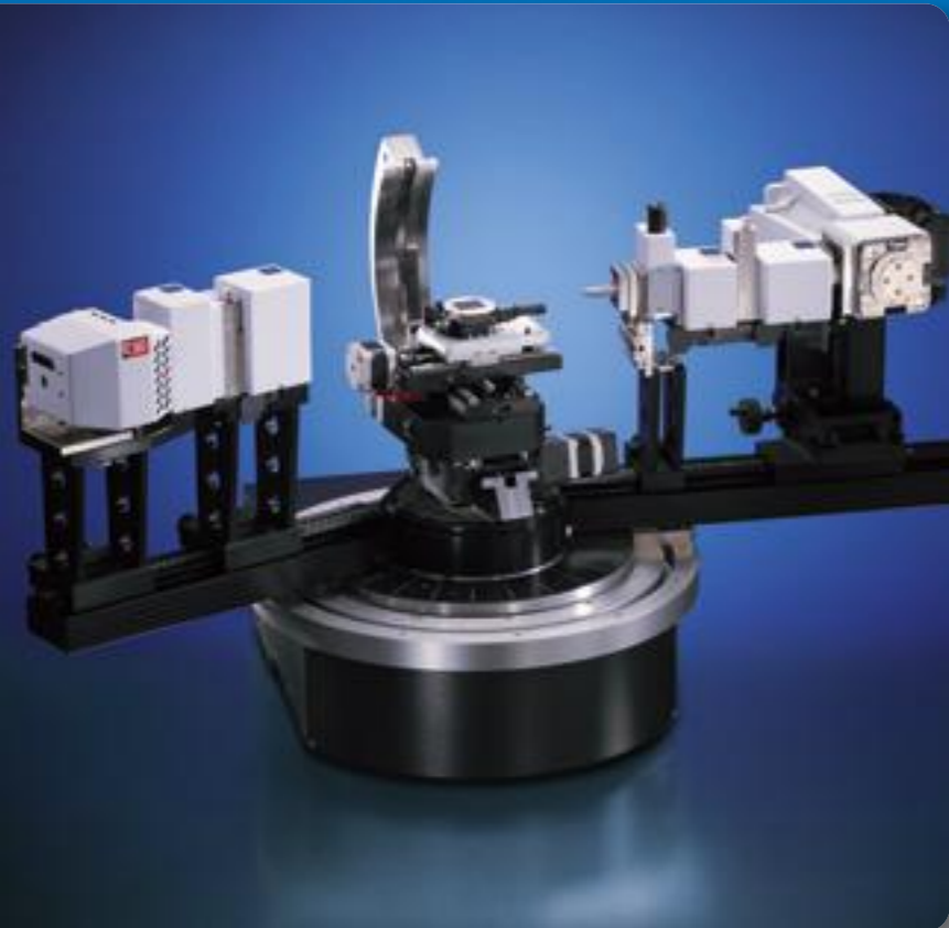
Grazing incidence diffraction setup with horizontal goniometer and Eulerian cradle
