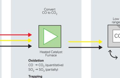
Long life catalyst ensures CO and volatile organic compounds are converted for a true total carbon result
